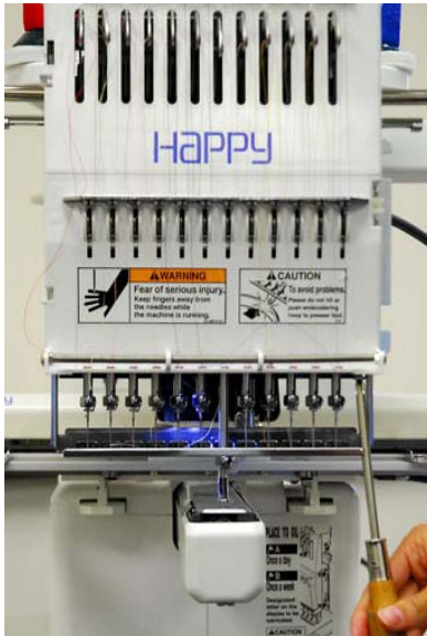
Remove the 2 screws along the bottom edge of the lower faceplate.
