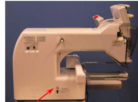
Press and hold after turning shaft to 90 degrees, then continue turning main shaft.
