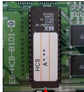
ROM chip inserted with notch facing downwards!
