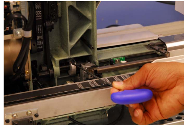
Turn shaft until this screw is visible and loosen with a 3mm hex wrench.
