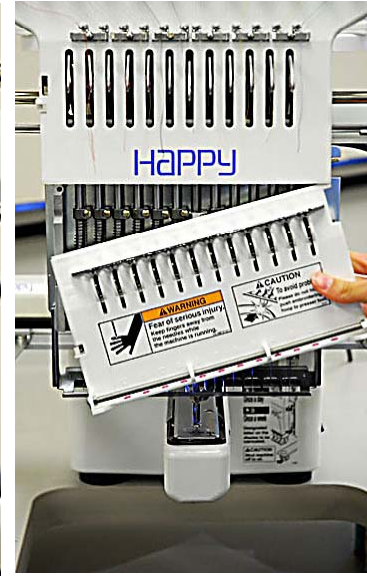
Careful – the lower faceplate will fall. Be ready to either hold the lower plate aside or leave unthreaded.
