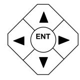
When machine is stopped, you can adjust the position of the design using a combination of the ENT keys and any of the arrow keys, which move the hoop and as a result the position of the design. (Note, you can permanently move this position by using the options available when holding MENU down, which is discussed in another document.)
