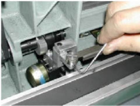
Figure 2.6a. Loosen this set screw with a 2mm hex wrench.
