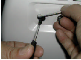
Remove the bobbin winder. Remove both the tensioning knob and switch arm.
