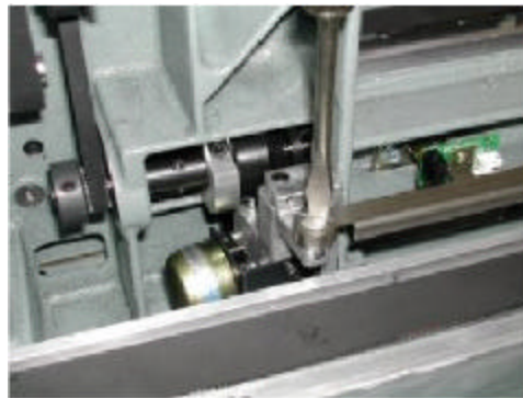
Figure 2.6b. Turn eccentric bolt until moving knife is positioned as shown in Figure 2.6c.
