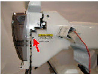
Remove 1 external and 2 internal screws. As shown above.
