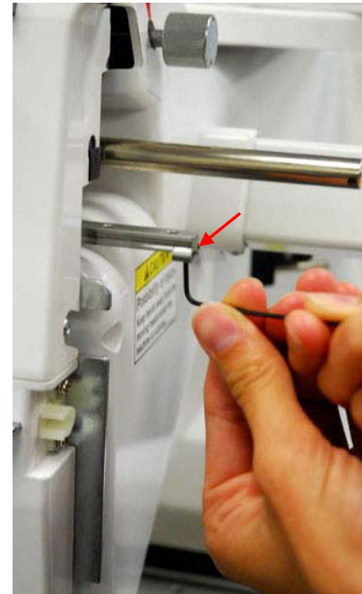
Remove this retaining clip with a 1.5 mm hex wrench.
