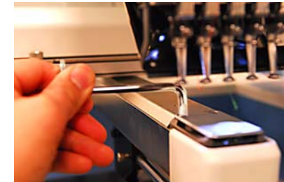
Remove the needle plate with an offset screwdriver as shown above.
