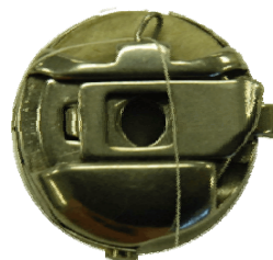
3. Pass thread under wire loop at the top front of the bobbin case.
