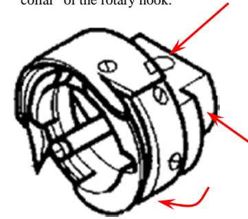
(side view) Turn the hook as necessary for easy access with a screwdriver.
