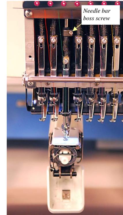
*(Left) with the lower plate removed, the needle bar boss screw is easily accessible for adjustment.*
