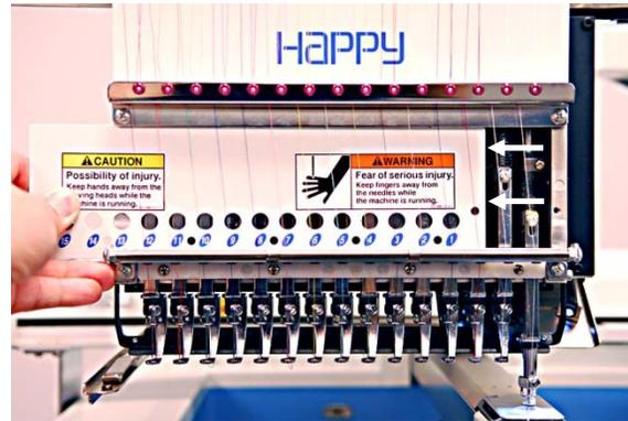
*(above) You can remove the lower faceplate by removing the 2 Phillips screws on either side. Caution: do not over-tighten these screws when replacing.*
