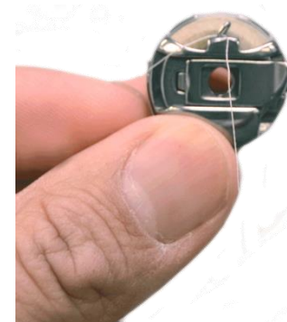
Figure 2: Make sure the bobbin is threaded like this (we will practice this in more detail in class) before inserting it.
