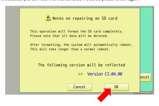
6. When "OK" is selected, the data on the SD card will be formatted and new data will be generated using the selected update package.
