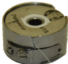
1. Ensure bobbin turns clockwise. Pull thread through this slit.
